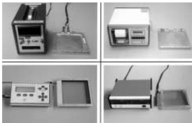
Fig. 1 Transmission chamber used in experiment. (a) Kyushu University type area/exposure Dosimeter (b) PTW Corporation's DIAMENTOR M2 area dosimeter (c) RTI Electronics Corporation's Doseguard 100 area dosimeter (d) TORECK Corporation's PD-4100 area/exposure dosimeter
