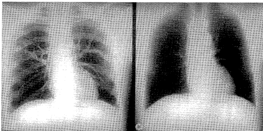
Fig. 7 Images of the chest phantom with a nylon nodule in the left upper lung zone. Left image is an original image and right image is a bone-subtracted image.
